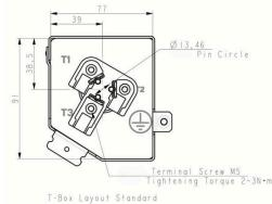
Application See Details in the YM serial MBP refrigerant scroll compressor application manual
